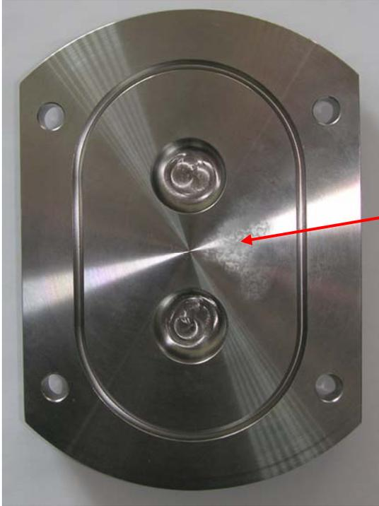
**Typical cavitation effect on pump rotorcase cover.**
