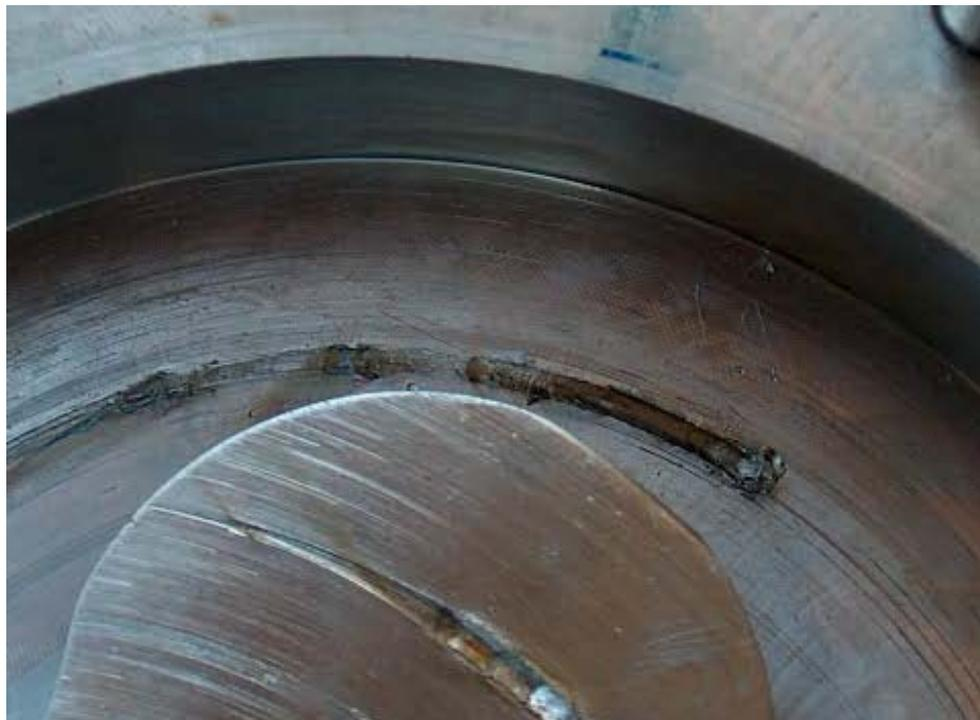
*Example of corrosion on pump rotor.*
