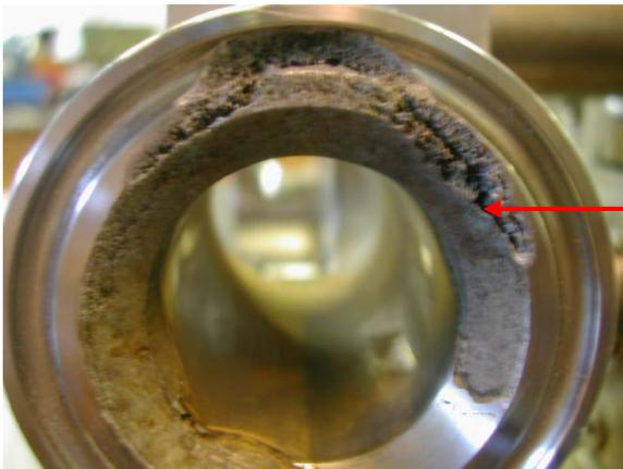
*Example of corrosion on pump rotorcase port.*
