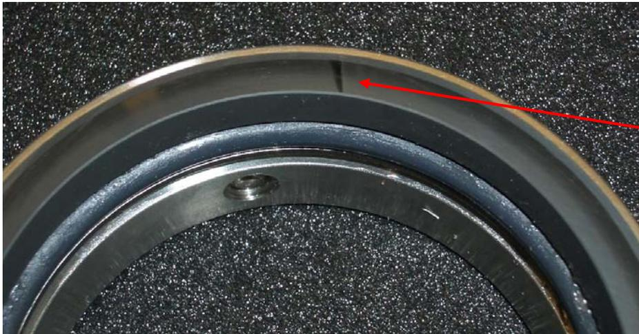
**Example of crack in seal insert caused by thermal shock**
