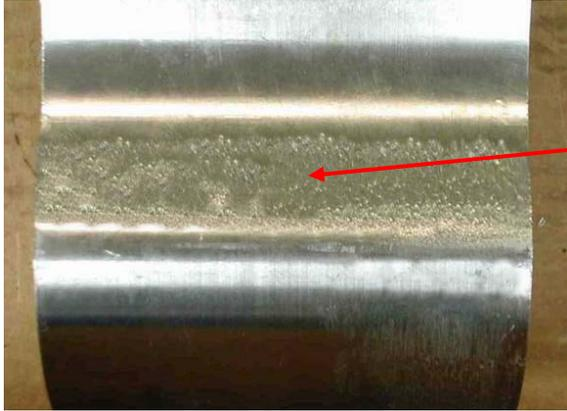
**Cavitation effect on pump rotor may result in rotor to rotor contact.**
