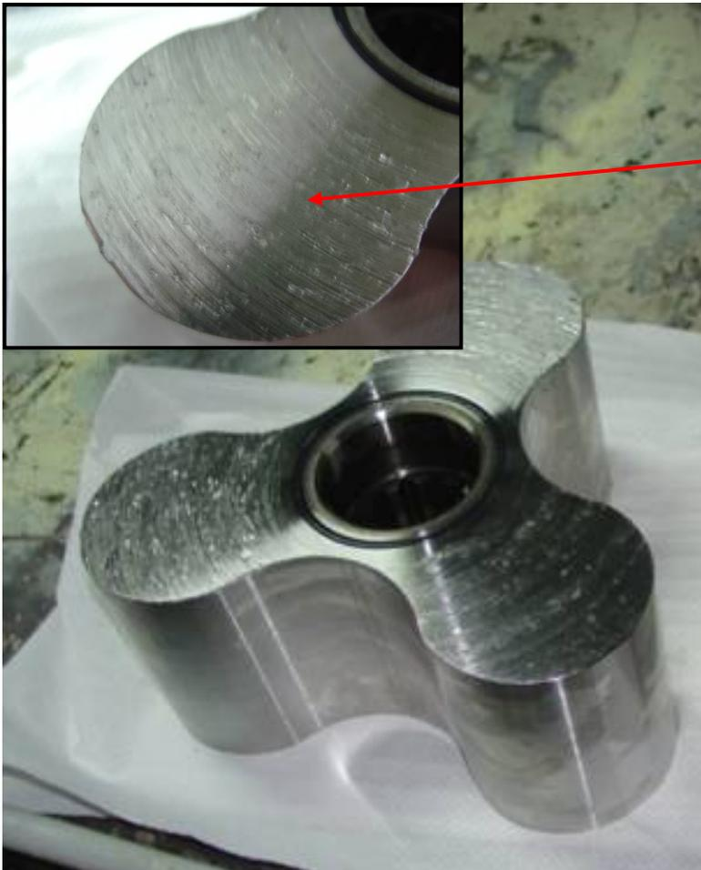
***Rear rotor face with signs of rotorcase contact, indicative of rapidly decreasing temperature i.e. thermal shock - hot to cold.***
