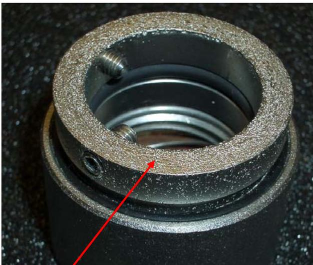
***Example of pitting corrosion on stainless steel***
