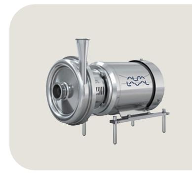
As standard, the LKH pump is equipped with a single mechanical shaft seal but is also available with a single flushed or a double mechanical shaft seal. The front-loading shaft seal, with the spring and washers mounted on the atmospheric side, makes maintenance fast, easy and inexpensive. It takes just a few minutes to replace the shaft seal. In addition, the balanced design minimizes the risk of seal opening during unforeseen pressure shock.
