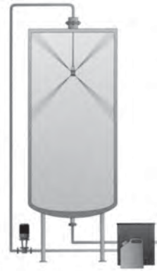
Minutes A full DIP pattern using high-impact rotary jet equipment from Alfa Laval is highly efficient and takes just a few minutes
