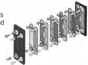
Flow principle of a plate heat exchanger
